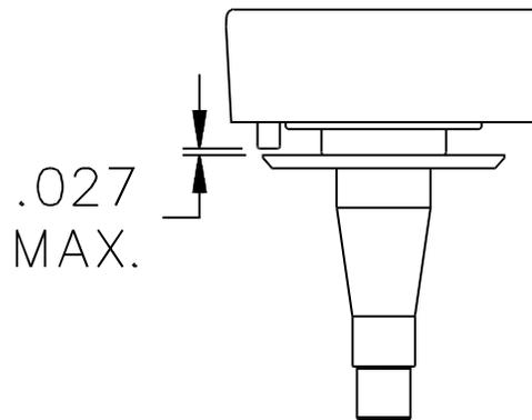
**Figure 7** - ABS Sensor and Tone Ring Gap
