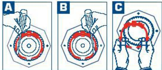
8. **A, B, C** Use a small screwdriver to carefully pry the keeper arm from the undercut groove on each side until the keeper is released.
