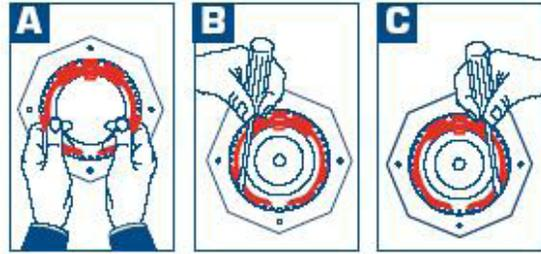
18. Compress and insert the keeper arms, one at a time, into the undercut groove with a small screwdriver.
