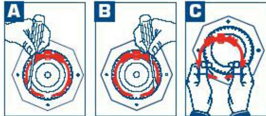
5. A, B, C Use a small screwdriver to carefully pry the keeper arm from the undercut groove on each side until the keeper is released.
