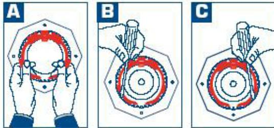
19. Compress and insert the keeper arms, one at a time, into the undercut groove with a small screwdriver.
