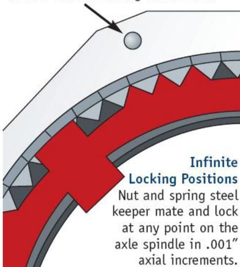
12. Adjust the bearing by tightening the nut to 100 ft-lb. Spin the wheel at least one full rotation.
