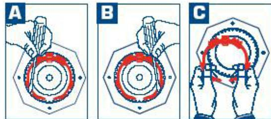
7. **A**, **B**, **C** Use a small screwdriver to carefully pry the keeper arm from the undercut groove on each side until the keeper is released.
