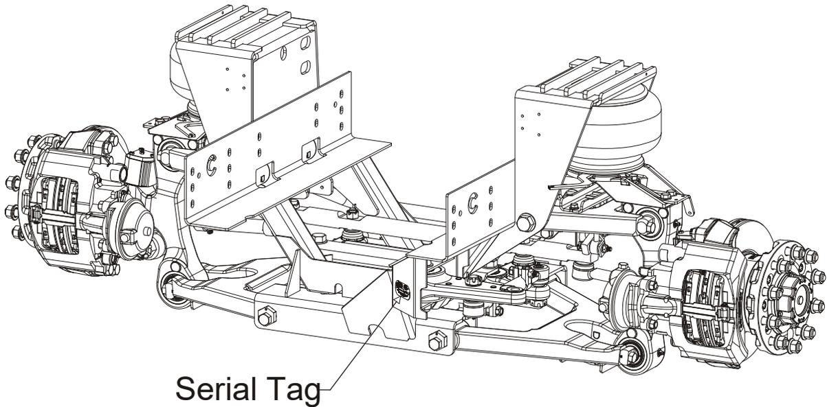
**Figure 1 - Suspension Identification Location**
