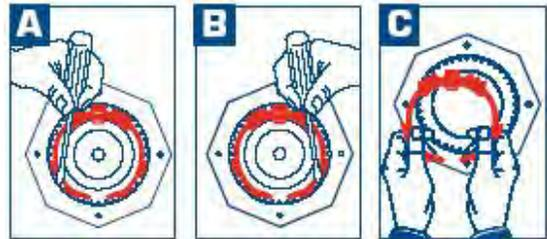
14. **A, B, C** Use a small screwdriver to carefully pry the keeper arm from the undercut groove on each side until the keeper is released.
