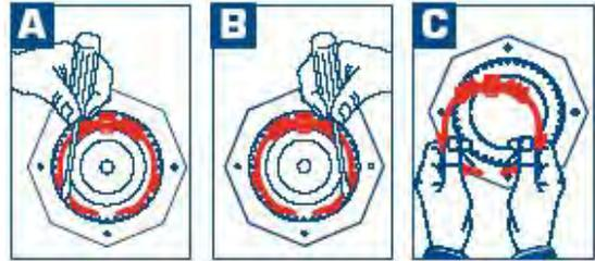
8. **A, B, C** Use a small screwdriver to carefully pry the keeper arm from the undercut groove on each side until the keeper is released.
