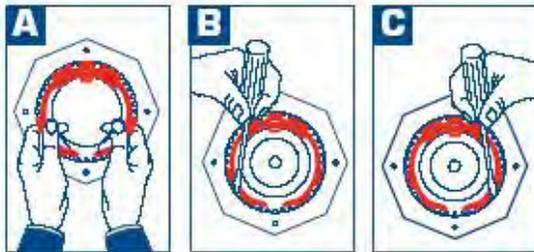
25. Compress and insert the keeper arms, one at a time, into the undercut groove with a small screwdriver.
