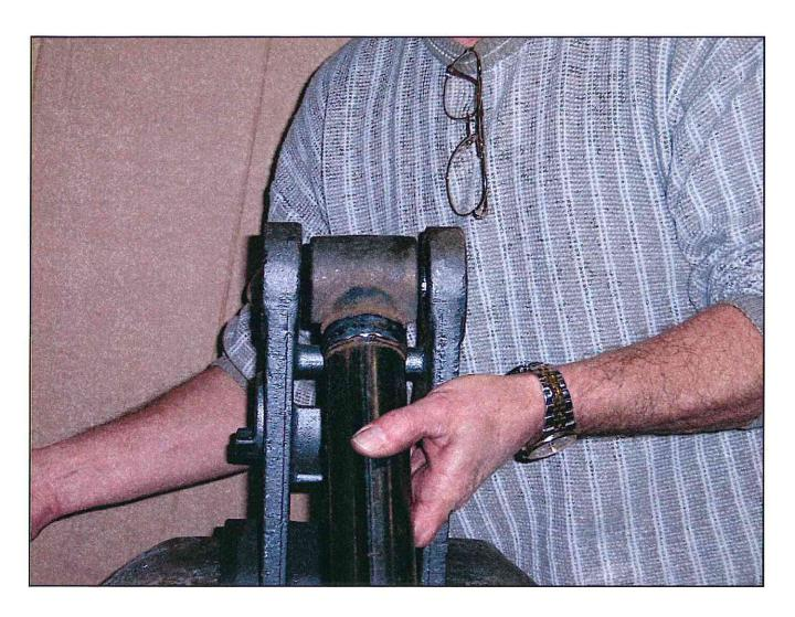
Center the torques arm between the ears of the suspension spring hanger.
